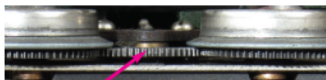
Gear side of a Type 9 motor. The arrow points to the single large gear that drives the gears mounted on the rear of the red, spoke drivers. The gear cover has a triangle shape.
