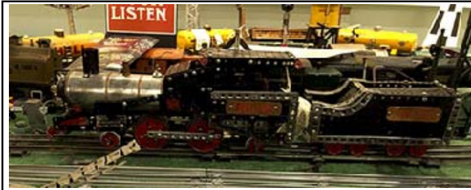
Erector set loco and tender. Rattle-can boiler. Power pickup in trailing truck. Erector motor inside cab loco. Chain drive. Hesitatingly runs/growls. Older build.
