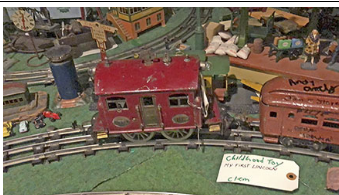
Snookins, a fav of mine, is a chopped Lionel #402 repainted in maroon. Her side panels are gone and the ends pieces soldered to the main body. Normally a twin engine, she carries a Lionel #38 motor, American Flyer steps and rearranged gingerbread. She runs very well and with a great attitude.
