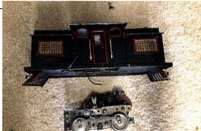
Sam, Son of STOMPER STG Yard engine History unknown. Motor modified IVES standing motor. Imbedded headlights.
