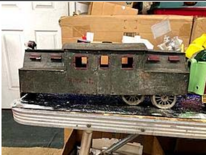
Body is tarnished tinplate. Motor is clock frame with 30 pitch gears. Builder used no frame, thus erector beams being installed.
