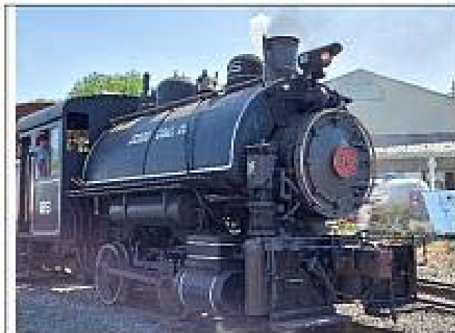
Tank engine with built in coal bunker
