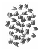
01-4000: DISTILLING COLUMN PACKING, PORCELAIN BERL SADDLES – Porcelain saddles having an OD of 6mm, ideal for vacuum distillation, absorption and extraction. Saddles provide a highly useable surface area, lower gas flow resistance and excellent internal distribution. Available in packages of 200cc and 1000cc boxes.
