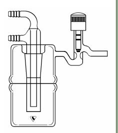
14-1060: SUBLIMINATION APPARATUS - For use in vacuum sublimination. Removable condenser allows for the introduction of alternate coolants into the well. Flask and condenser seal together with an o-ring connection. A 4mm Teflon valve controls the vacuum.
