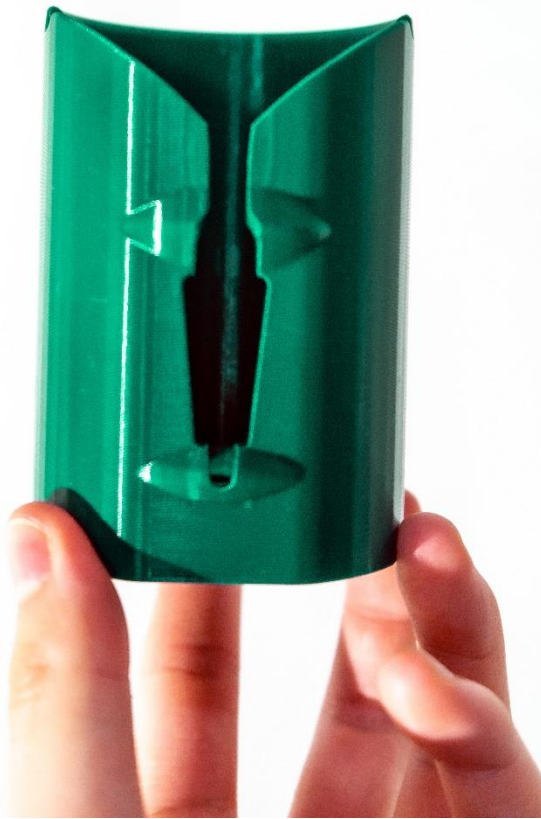
Figure 4. DECAP functional piece prior to SLA inserts, printed on Creator 4 Pro
