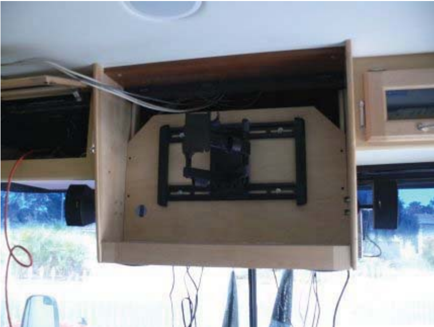
New bulkhead in front of woofer with adjustable TV mount.
