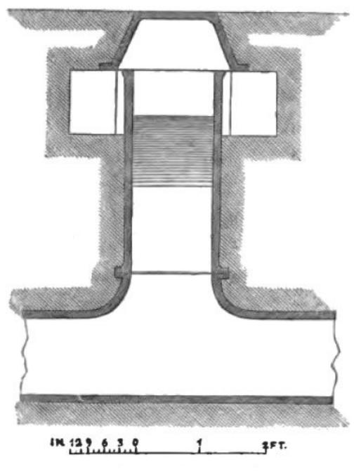
Fig 6. Opening for Suction-pipe.
