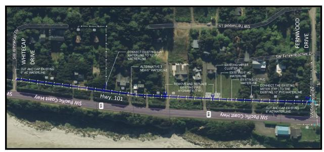
Figure 8 - East Side of Hwy. 101 Waterline Site Improvement Layout
