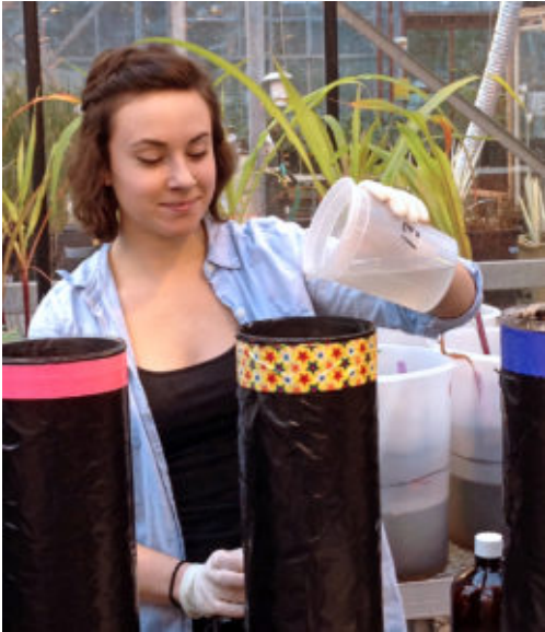
Megan Tyler-Plog pours collected storm water into a biofiltration strip soil mixture at University of Washington lab to measure nutrient and metals removal.
