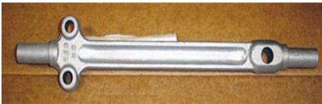
This early lower control arm shaft was used reportedly until 1964. Lower control arms manufactured before December 4, 1962, were part numbers 3817549 and 3817540. Later lower control arms were part numbers 3840603 and 3840604 with additional support bracket for the sway bar. This is where verification of correct pieces can become difficult, with the lower control arm shaft being used in both the early and late lower control arm.
