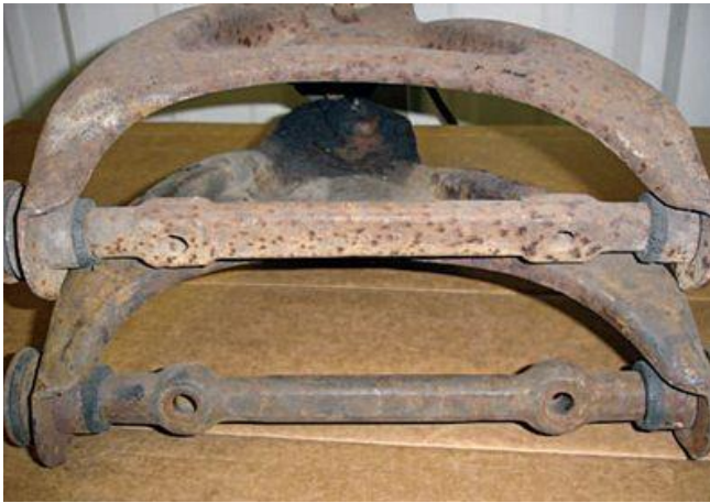
The 1963-1966 control arm (top) is an early upper control arm with rectangular control arm shaft. The late 1966 through 1982 production upper control arm (bottom) has a round control arm shaft. This is one of many things you need to know for an NCRS or Bloomington Gold restoration
