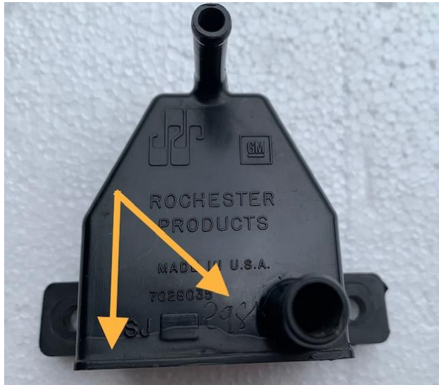
Fig. 2- Original valve note the added sealant and hand engraved number
