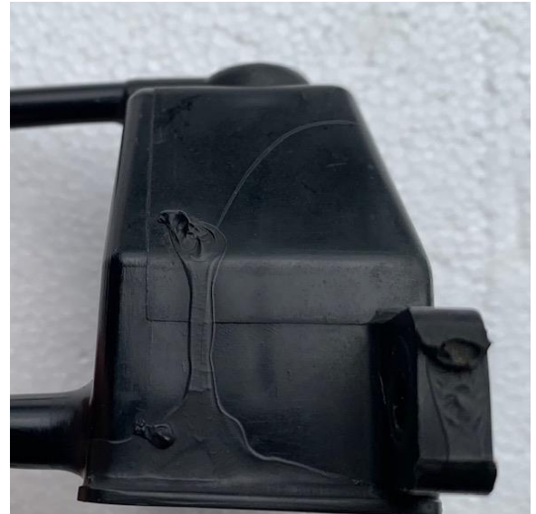
Fig. 3- Original Valve side view...note the extreme amount of sloppy factory sealant
