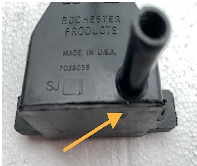
Fig. 4 – Repro common bottom seam failure
