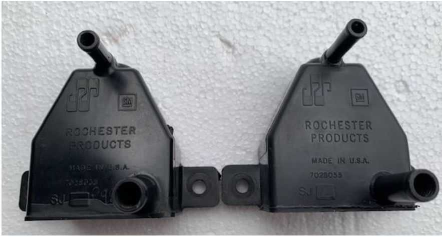
Fig. 1- Original valve (Left) Reproduction valve (Right)
