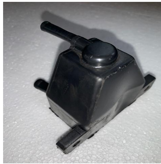
Fig. 5 – Repro collapsed valve
