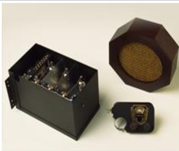
This reproduction of Motorola's first car radio, 1930's model 5T71, included (left to right) a radio receiver, tuning control and speaker.
