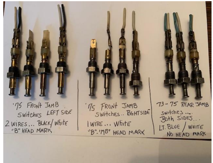
Fig. 8 Note the different colored wires used.
