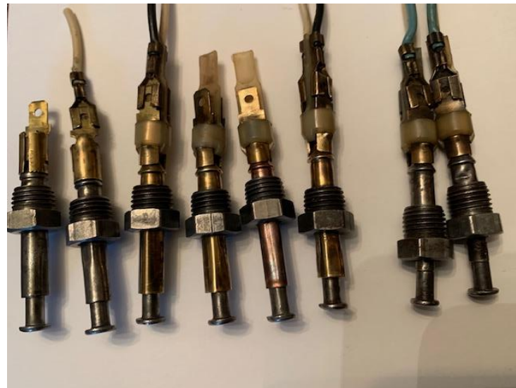
Fig. 5 – The many variations in spade-style switches. The two on the far right are the under-hood alarm switches from a 73. Note the solder drop on the last switch to keep its adjustment.
