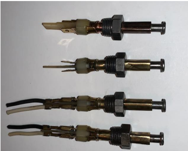
Fig.3 Note the differences in the metals used in these switches. The top switch is a great example of the crimped barrel.
