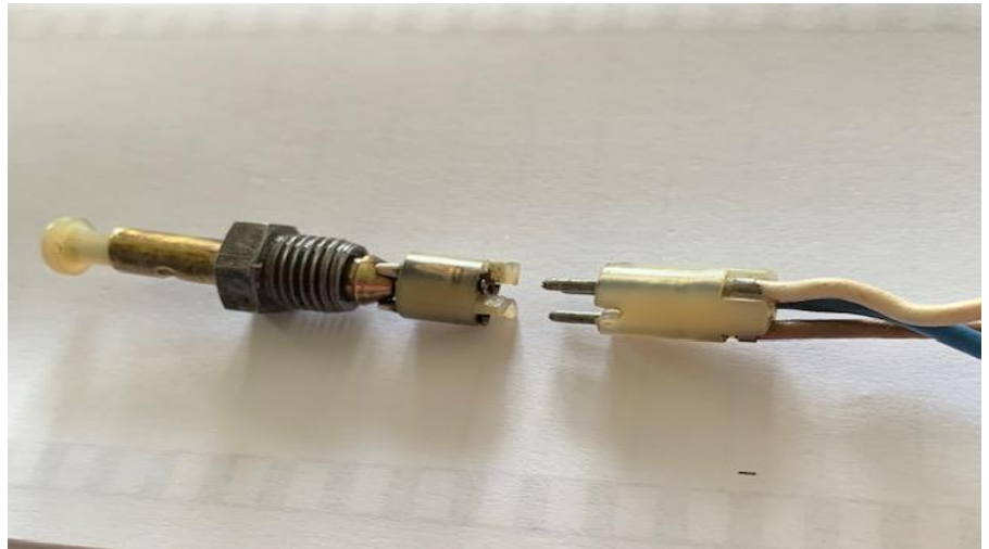
Fig. 9 This is an example of the front jamb switch from a 78-79. Note the change once again in the connection. No longer is the spade or pin style connection used. (Photo below 75-77 head closeup view!)
