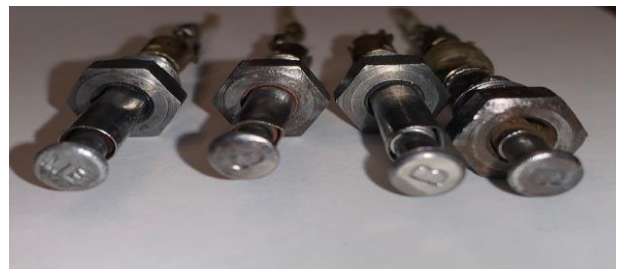
Fig. 9 This is an example of the front jamb switch from a 78-79. Note the change once again in the connection. No longer is the spade or pin style connection used. (Photo below 75-77 head closeup view!)
