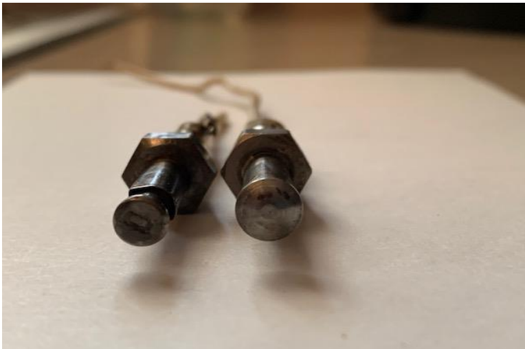
Fig. 6- later thru 76 head & plunger size change. Note the larger head on the right.
