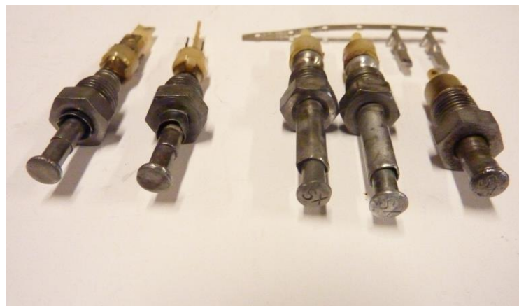
Fig. 1 -73-74 switches Spade-style on left, pin style on right. Note no head marking on the rear spade switches. SX visible on front jamb switches. Switch to far right is one from under the hood. Note the smaller size. The item at the top right is an example of the replacement pins and how they come from the vendors.
