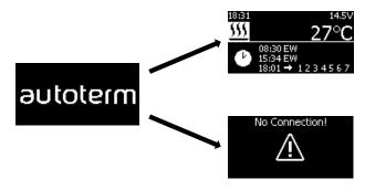
After disconnecting the control panel form the power supply time and date must be reset. Rest of the settings, such as set timers, remain saved.
