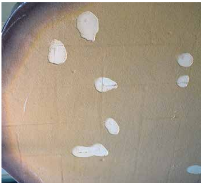
Remove loose chips from lid and replace crumbling lids to prevent chunks from falling on ware during firing.
