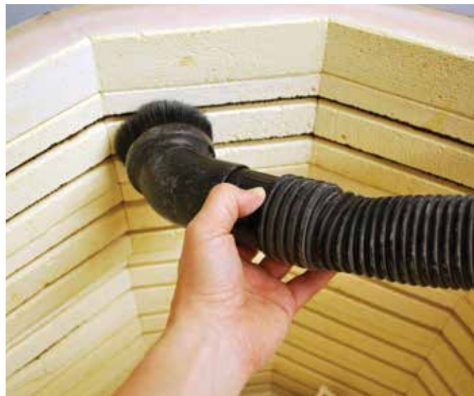
Use a soft brush attachment to vacuum the interior of the kiln.
