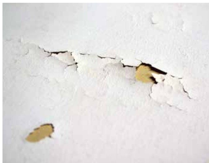
Remove loose, flaking kiln wash from shelves and recoat them.
