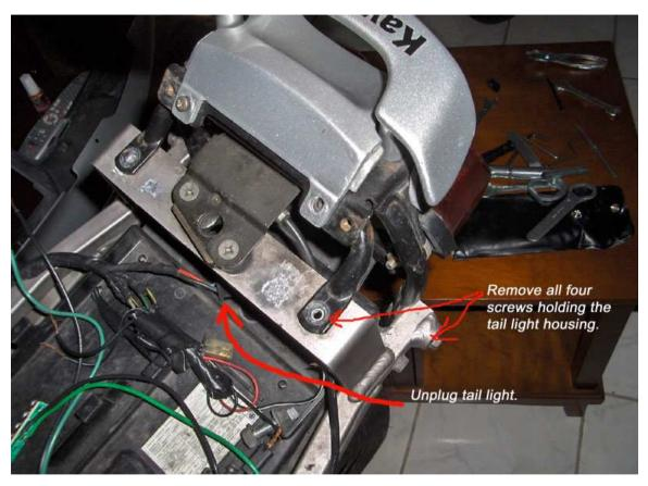
Start by removing your entire tail piece, including the tail light housing. It is a total of 3 parts: The two sides and the tail light housing.
