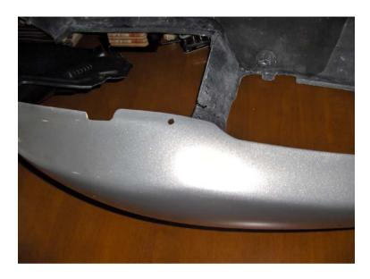
Now that the tail piece is put together outside the bike, take a very small drill bit (between 1/16th and 3/32nd its fine) and make the four holes in the same places shown below:
