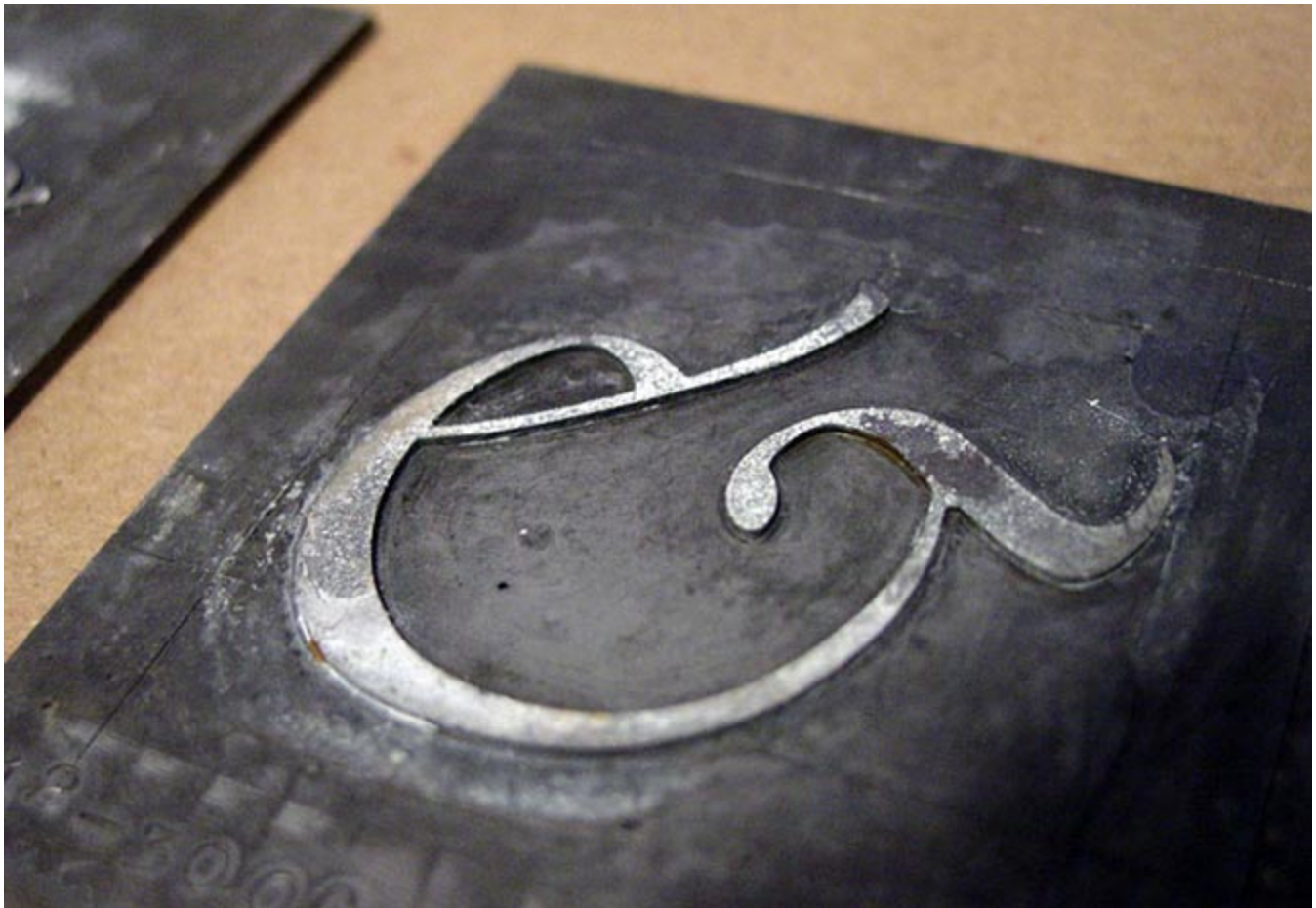
The original Lanston-Monotype patterns were used as source material for Californian . Shown here is the ampersand (&) for the Italic.
