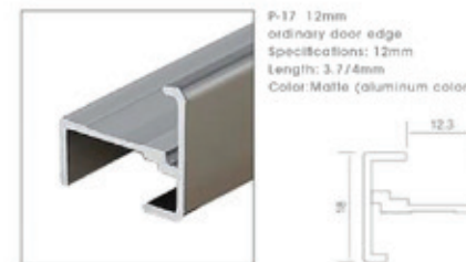
P-17 12mm ordinary door edge Specifications: 12mm Length: 3.7/4mm Color:Matte (aluminum color)
