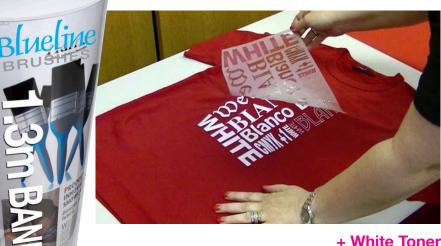
Historically, printing solid white on to media has always proved to be a challenge for digital print devices. Printing white text or graphics has been limited to either using white media or the slow and costly process of litho/ screen printing. The launch of the Intec ColorSplash CS5000 provides an affordable, easy to use alternative.
