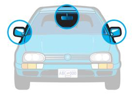
Most cars have three mirrors to help you see what's going on around your vehicle. Some cars do not have an outside mirror on the passenger side.
