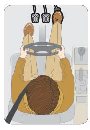
You will operate two or three controls with your feet, depending on whether your vehicle has an automatic or a standard transmission.
