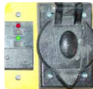
Figure 5 GFCI Circuit Model on the left and the outlet on the right.
