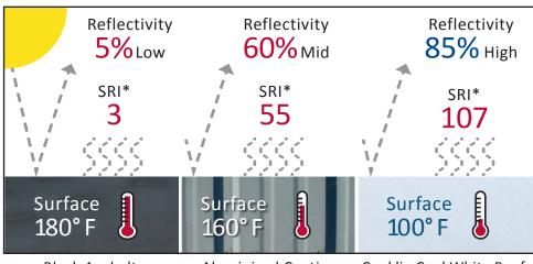
\*The Solar Reflectance Index (SRI) is a measure defined by the Lawrence Berkeley National Laboratory as the roof's ability to reject solar heat, as shown by a small temperature rise. It is defined so that a standard black (reflectance 0.05, emittance 0.90) is 0 and a standard white (reflectance 0.80, emittance 0.90) is 100. Due to the way SRI is defined, particularly hot materials can even take slightly negative values, and particularly cool materials can even exceed 100.
