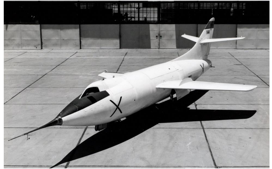
Douglas D-558-2 high-speed canopy, All-rocket Propulsion Air-launch from Boeing P2B-1S
