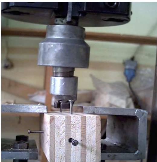
Fig. 5. Experiment set-up for nail withdrawal.
