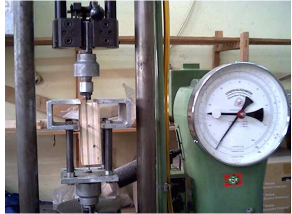
Fig. 6. Experiment in transverse surface and set-up of radial surface.
