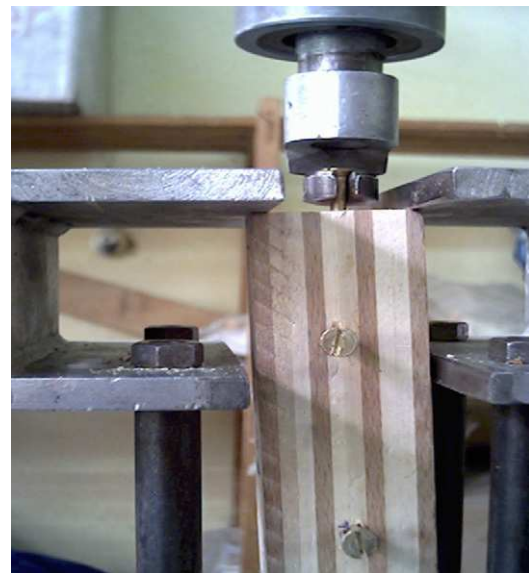
Fig. 3. Experiment set-up of PVAc5 tangential surface and test of poplar–poplar intersection in transverse surface.
