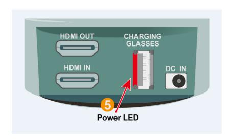
The 5 power LED will glow red when in use. When the power cable input the power LED will quickly turn on, then BLINKING and waiting receives HDMI signal transit, and then on permanently to indicate that the 3D Edison handshake has been completed.
