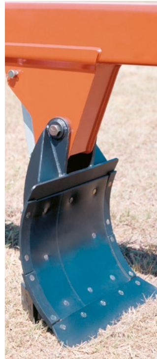
Moldboard with plastic lining
