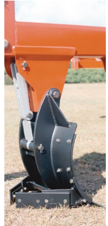
Moldboard trip system with flat spring
