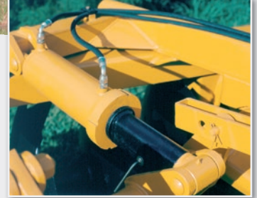
Hydraulic cylinders with hoses and quick couplers.
