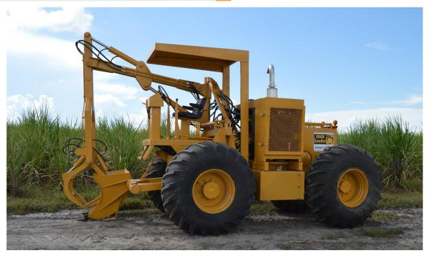
**Engine:** John Deere 4045T Engine 105 continuous HP @ 2200 RPM, 116 RATED HP @ 2200 RPM
