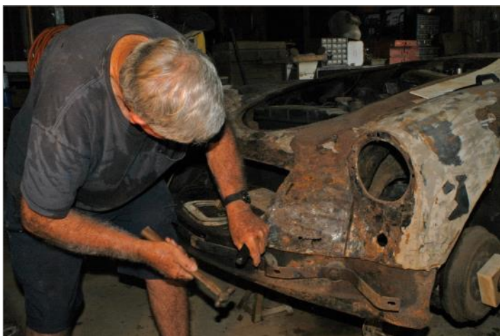
Old botched fiberglass repairs are removed with a hammer and screwdriver.
