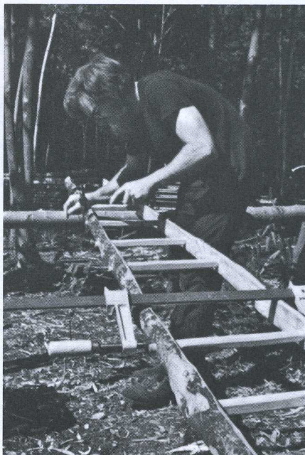
After the first rail has been completely nailed, draw in the other rail tightly with either a pipe vise or clamp and nail the rungs into it.
