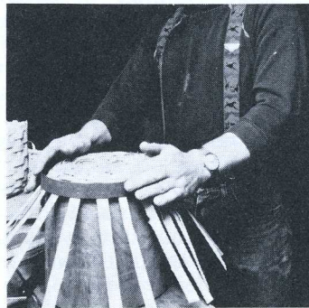
1. After loosening the wood with a mallet, Colburn lifts off the peel in annual layers. 2. He strips the peel with a device having a row of razor blades embedded in the top at one-inch intervals. 3. The base is woven on a low conical block. 4. The woven base is then reversed and set on the concave end of the basket mold. A metal hoop keeps the stave ends close to the mold. 5. A metal bar inserted into one end of the mold is clamped in a bench vise. This allows Colburn to rotate the mold at an adjustable angle. 6. Shaving a wood strip for a single-handle basket.
