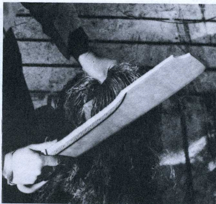
Figure 10-3. Scutching broken flax against a scutching block with a carved wooden scutching knife.
