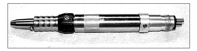
The Champion Little Guy 5K Motor is used mainly by dental hygienists. Typically a prophy cup is inserted in the nose portion and tightened using the chuck collar. The motor is equipped with a forward and reverse ring allowing dual direction spin. The repair on this motor is similar to a Star 5K or 20K motor. As always, try to determine the problem with the handpiece before disassembling the motor.
