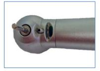
Notice that the KaVo 646B has a Glass Fiber Optic Rod and a single port water spray. If there is a water problem, you can try clearing it with your Smart Cleaner tool, (part# 00082) or you can use a small thin wire to dislodge any debris.
