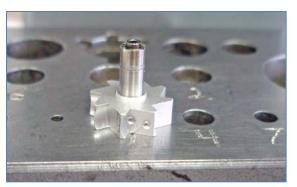
**STEP 1 Original Turbine Only:** Place your impeller over Hole #1 in your work block as shown at left. Then, manually slip the front of the spindle down into the impeller.
