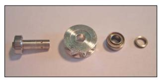
You should now line up your new assembly as pictured at left. Spindle with bearing, Impeller, Front Bearing and Slinger Washer
