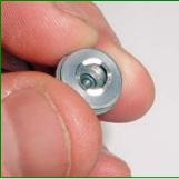
**STEP 6 Original Turbine Only:** Place the o-ring into the back cap. Secure it into the groove as shown (far left).
