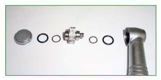
**Original Turbine Only:** Please line-up your 659B Turbine assembly as pictured at left. It should consist of a Back Cap, 2 – O-rings, 2-Loading Springs, the now assembled Turbine and the Handpiece.
