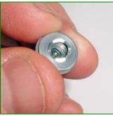
STEP 5 After-Market Turbine Only: Place the o-ring into the back cap. Secure it into the groove as shown (far left).
