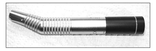
This Kavo LN motor is slightly newer than the Kavo L models. It features a cellular optic rod as opposed to the old fiber optic bundles that tend to go bad quickly. As a result, the repair procedure requires more care but is easier as a whole. The repair procedure below will be using a 2307LN motor but the repair on this motor is very similar to that of the 2320LN, 2329LN and 2325LN motors. As always, try to determine the problem before disassembling the motor.
