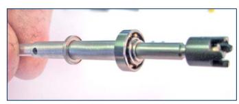
After the C-Clip is inserted, Slide the Lower Bearing Spacer onto the shaft.
