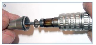
The Bearing Spacer has a raised lip on its outer edge. This lip rests against the Bearing.
