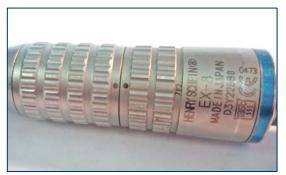
Now secure the Bottom Nosecone Housing to the Middle Nosecone Housing. Tighten the two together but STOP when the two Chuck Indicator Dots align.
