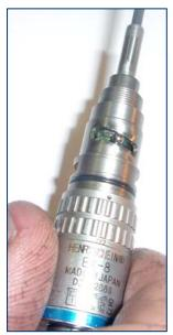
Place a dab of grease in the Collet Opener and slit (Pictured Below). Next, place one of the Chuck Balls into the slit (Pictured at Left). It will be held nicely by the grease. Turn the nosecone exactly 180 degrees and place the second Chuck Ball in the other slit. Make sure the Chuck Balls are exactly opposite of each other.
