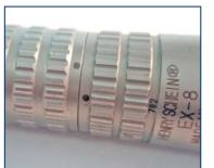
Notice in the picture at left, that the Chuck Indicator Dots are not lined up properly. The lower Dot has passed the upper Dot during the tightening process.
