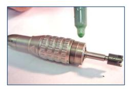
The solution is simple. Unscrew the Bottom Nosecone Housing from the Middle Housing. Place a small drop of LocTite onto the threads. The picture at left is an example of Too Much LocTite, simply shown to distinguish what we are doing. In practice, it is safer to put a small drop of LocTite onto a pin or needle and apply it to the threads in that manner.
