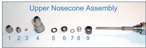
STEP 4 Carefully lay out the loose pieces that were exposed when you removed the upper nose housing.
