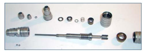
**STEP 6** Once you have removed the 2 Chuck Balls from the angled groove they rest in, place the front of the nosecone into a 21/32"
