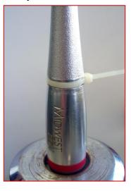
carefully lower the nose section onto the motor assembly, which should be secured, once again in a 9/16° collet.
