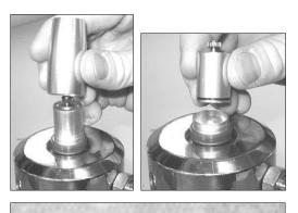
Now place the threads of the motor into a 9/16" collet (far left picture). Remove the motor housing by unthreading it in a counterclockwise direction. Place the outer housing on your work surface and then remove the motor canister from the base piece (near left picture). It should simply lift out with little resistance.
