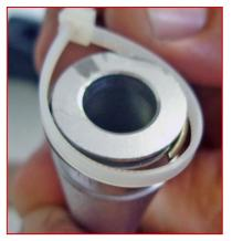
Now we must connect our reassembled nose section to the main RDH Body. First, secure and compress the large C-Clip at the bottom of the nose section with a large Zip-Tie, (larger ones work best).
