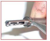
To remove the small brass clip washer, take your exacto knife and carefully slip it out of its groove. Then, slowly slide it up and off the end of the chuck.
