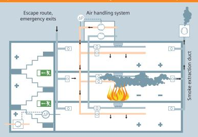
Ventilation systems must switch off independently when fire alarm or extinguishing systems are activated and when thermal cutout devices of the fire and smoke protection dampers are activated, or switch from normal to emergency operation. This operating mode ensures, for example, that the rooms are systematically regulated for overpressure so that escape routes remain free of smoke.
