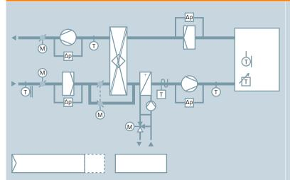
Demand-based operation of ventilation plants ensures energy-efficient ventilation. Depending on the requirements and type of plant, important plant elements that must be activated in an energy-optimized manner are outside air, exhaust air, recirculated air or bypass dampers. OpenAir damper actuators satisfy these requirements precisely and reliably.
