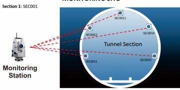
Total Station will take measurement of the prisms from the lower left to right or from Prism 1 – 5 of the section
