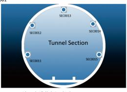
Prism are installed in the Tunnel Sections
