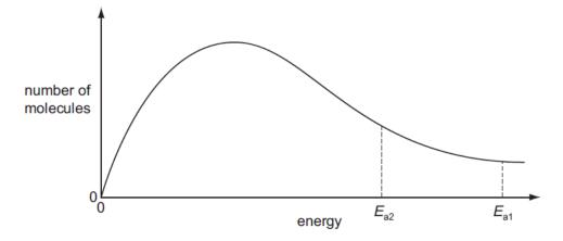
$E_{\rm a}$  is the activation energy for the reaction between the gases. Of the two values shown, one is for a catalysed reaction, the other for an uncatalysed one.
