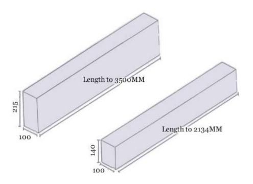
All Hampton Cast Stone lintels are reinforced for self – weight and handling purposes and for structural (load bearing) use.
