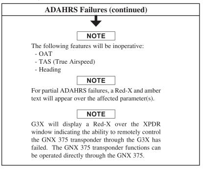
After a brief delay, the G3X will display attitude, altitude, and airspeed information from the G5 standby instrument as indicated by AHRS REVERT and ADC REVERT amber CAS messages. The G3X and G5 standby heading will be inoperative requiring the pilot to use the non-stabilized magnetic compass or other information for course guidance. See Section 3.1 for additional information concerning PFD alerts.
