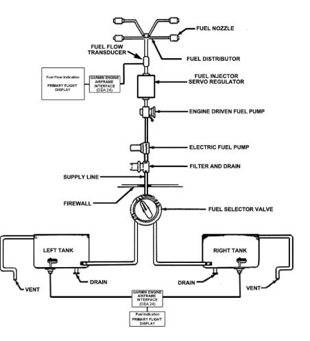
FUEL SYSTEM SCHEMATIC - Fuel Injected Engine -Figure 7-13
