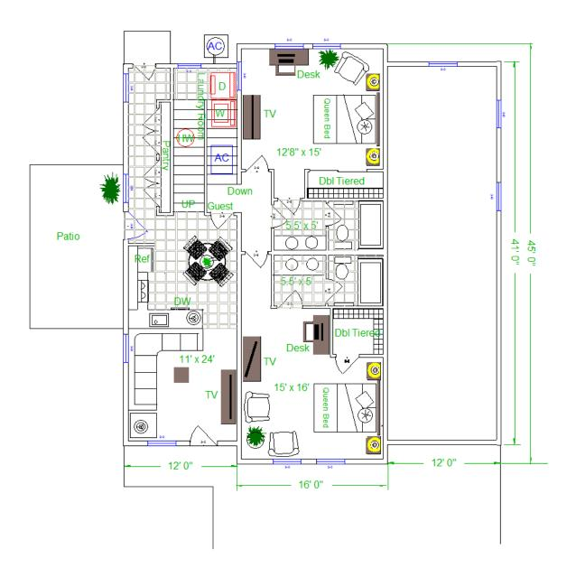
Floor plan is based on the foregoing models; however, the RV bridge has been shortened from 20' in width to 16' (the pricing below is for a 20' wide RV bridge). The way in which the staircase is designed allows room for a washer and dryer, hot water heater, and AC blower.
