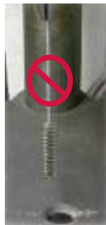
Incorrect Mounting in Chuck
