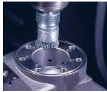
Blending tool marks on a hydraulic component.
