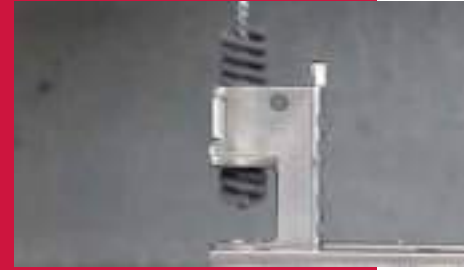
Deburring cross holes in a firearms component.
