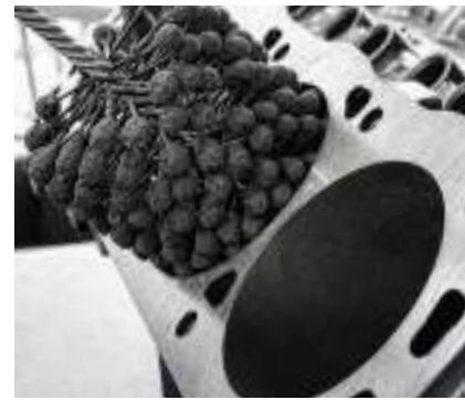
Engine cylinder head honing.
