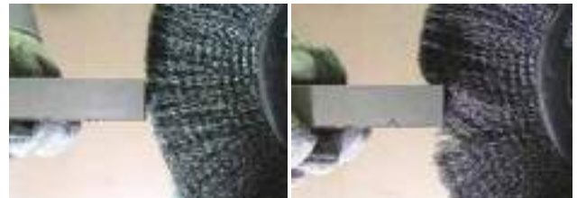
Correct Wire Tips Doing the Work
