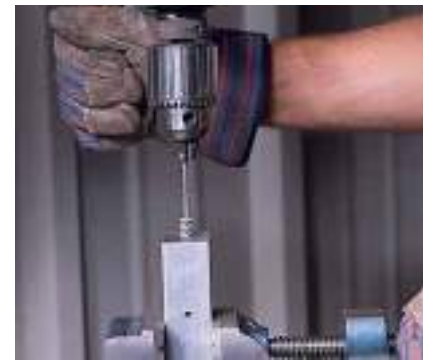
Crosshole deburring an aluminum manifold.
