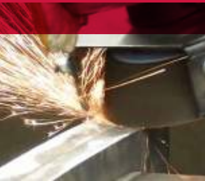
Type 11 Cup Rock for snagging and heavy stock removal.
