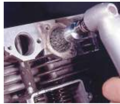
Cleaning the exhaust port of a gasoline engine.
