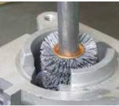
Deburring internal bores of a cylinder head.
