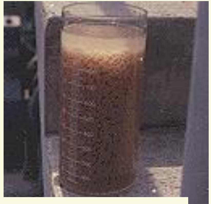
Raven Settleometer with curdled (Goldilocks) floc
