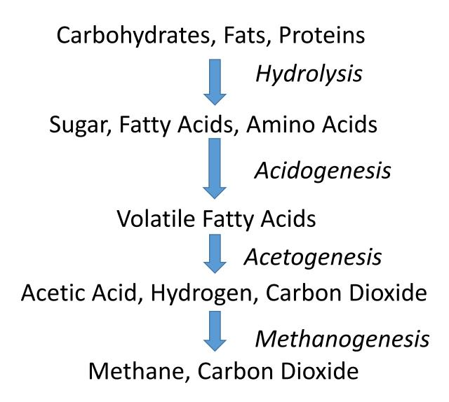
The performance of anaerobic digestion in destroying volatile (organic) matter to methane and carbon dioxide depends on:
