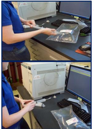
Gas can be tested onsite using a gas chromatograph or sent via tedlar bag (shown above) or cannister to outside lab
