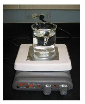
2. Place beaker on magneticspinner and add magneticstir bar. Adjust to slow speed.
