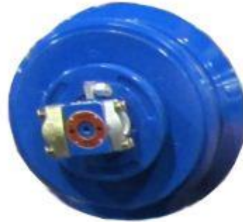
2080-D Rotodiff Weight: 170kg/375lbs Torque: 25,400Nm
